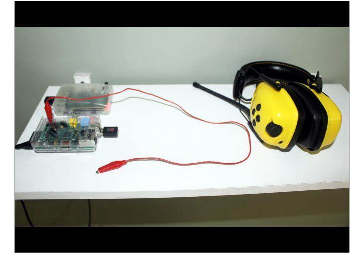
HouseFM is an on-site installation consisting of multiple raspberry pis broadcasting a unique soundscape over a shared FM channel, which was set to 90.1. As participants move throughout the house wearing FM radio enabled headphones, the audible signal from each Raspberry Pi will fade in and out as you move towards and away from each station.
