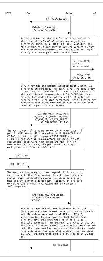
Figure 2: EAP-AKA' FS Authentication Process
