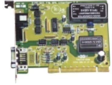
Interface board for the Trimble GPS receivers, developed in collaboration with NIKHEF
